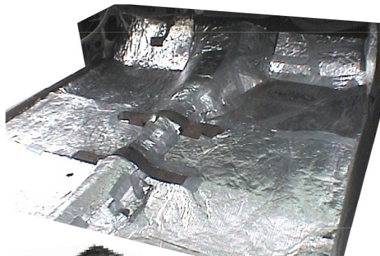
Pre-trimmed heat shield
