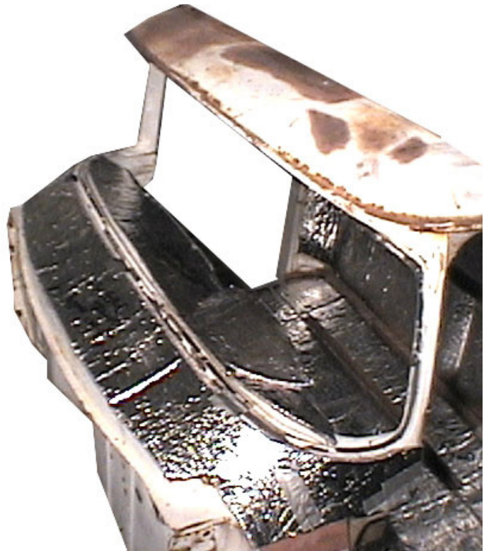
Cowl Absorber Panel ready to tape.
