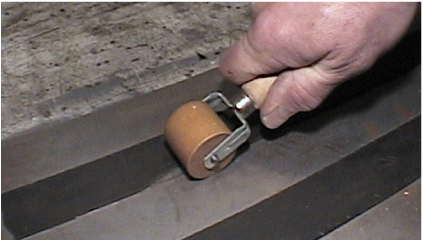
Placement of Door Skin Damper Strips on Cars and Trucks where access to the door skin is not limited by the internal door structure.
