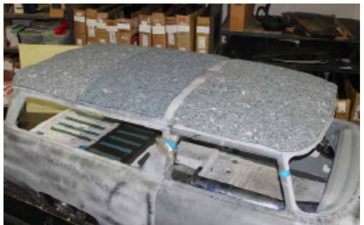
Typical Roof Panel Sound Dampening and Thermal Barrier Insulation.
