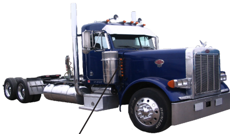
Cowl Kit Panels between the firewall and front door of the vehicle
