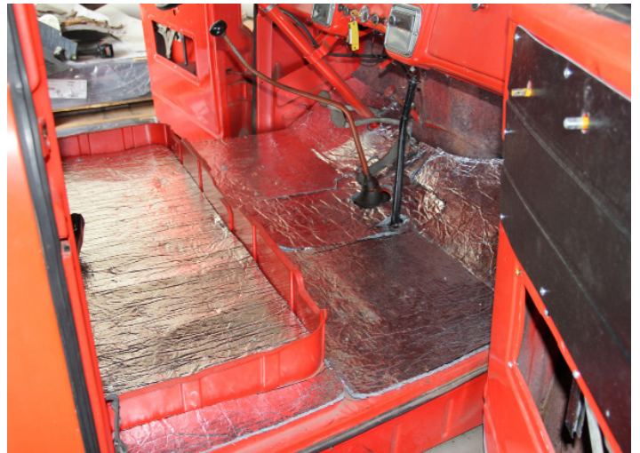
Typical Floor Panel Sound Dampening and Thermal Barrier Insulation.
