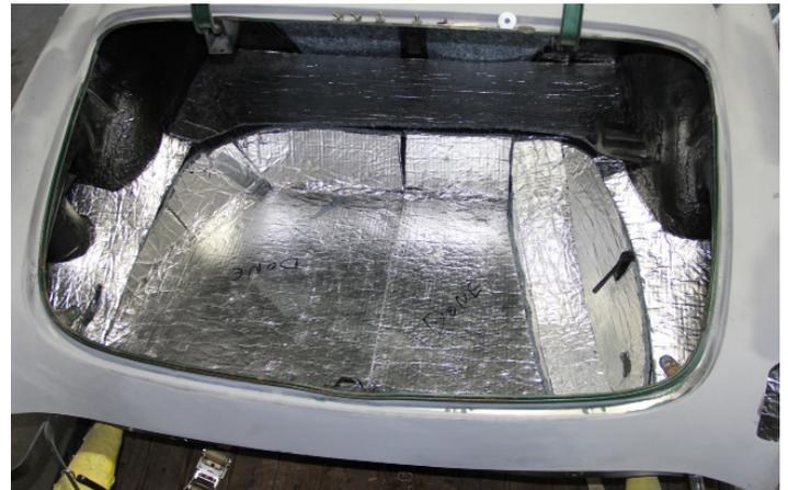
Typical Trunk Floor Sound Dampening and Thermal Barrier Insulation.
