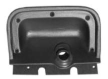
The Firewall bulkhead in many of the Post -War Chrysler, Dodge, DeSoto and Plymouth cars was commonly shared across production lines with the addition or deletion of a hole here and there to accomodated brand specific engines and accessory equipment.
