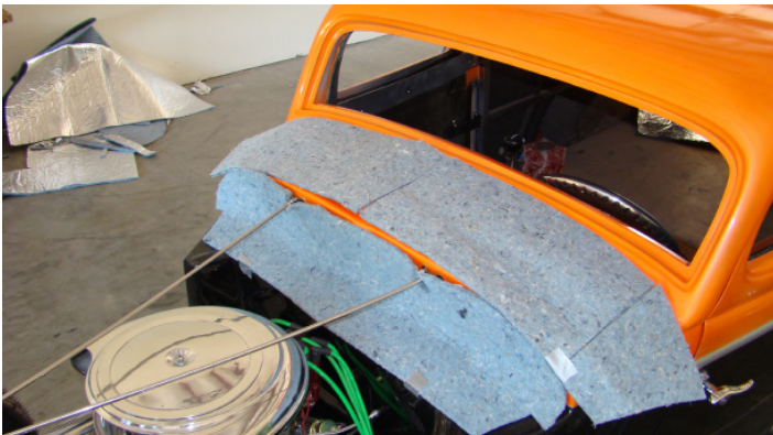
Typical Cowl Panel Sound Dampening and Thermal Barrier Insulation.
