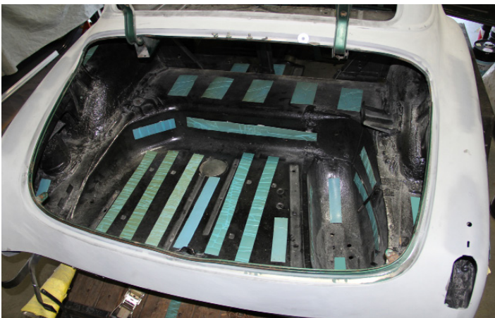
Typical Trunk Floor Sound Dampening and Thermal Barrier Insulation
