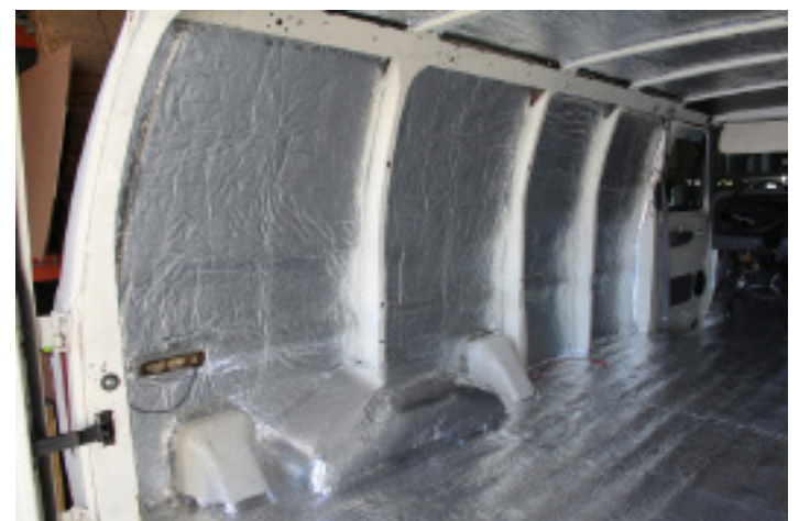
Typical Body Panel Sound Damping and Thermal Barrier Insulation
