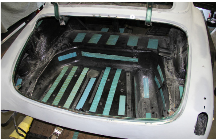
Typical Trunk Floor Sound Damping and Thermal Barrier Insulation.
