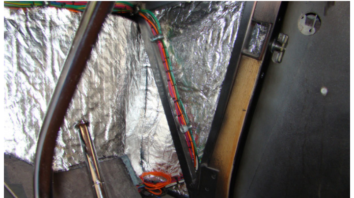
Typical Cowl Panel Sound Damping and Thermal Barrier Insulation.
