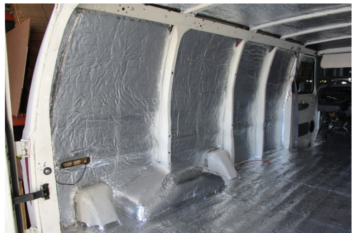
Typical Body Panel Sound Dampening and Thermal Barrier Insulation.
