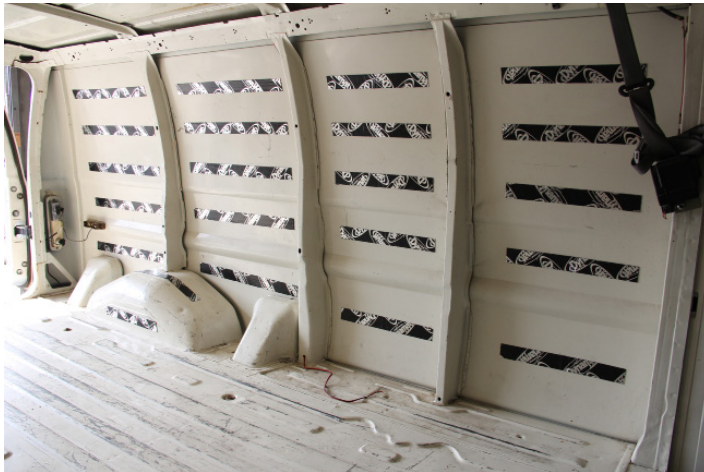
Typical Body Panel Sound Dampening and Thermal Barrier Insulation.
