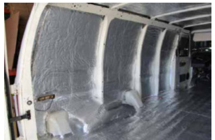
Typical Body Panel Sound Dampening and Thermal Barrier Insulation.
