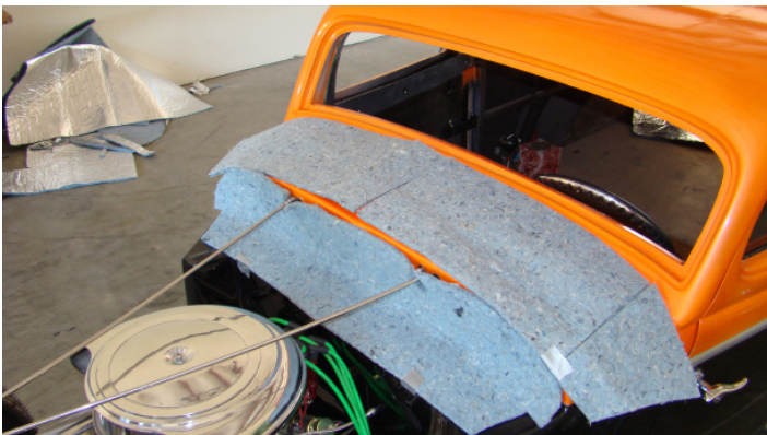
Typical Cowl Panel Sound Dampening and Thermal Barrier Insulation.
