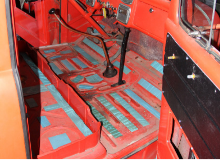
Typical Floor Panel Sound Dampening and Thermal Barrier Insulation.
