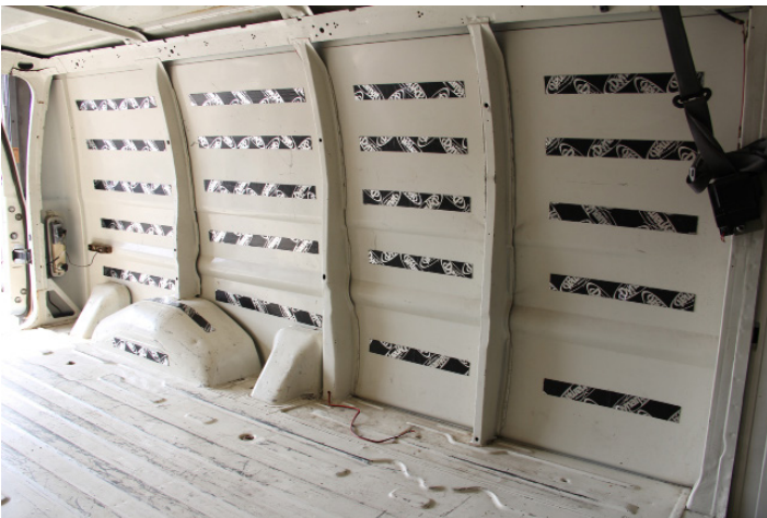
Typical Body Panel Sound Damping and Thermal Barrier Insulation.
