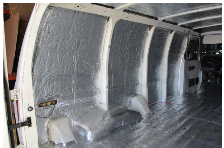
Typical Body Panel Sound Damping and Thermal Barrier Insulation.
