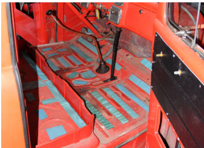
Typical Floor Panel Sound Damping and Thermal Barrier Insulation.
