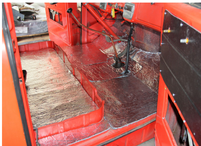
Typical Floor Panel Sound Damping and Thermal Barrier Insulation.
