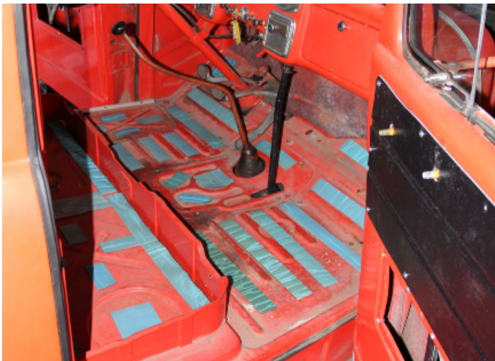
Typical Floor Panel Sound Dampening and Barrier Insulation
