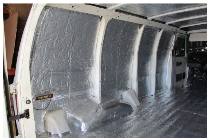
Typical Body Panel Sound Dampening and Barrier Insulation
