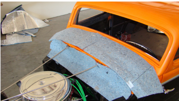
Typical Cowl Panel Sound Dampening and Barrier Insulation
