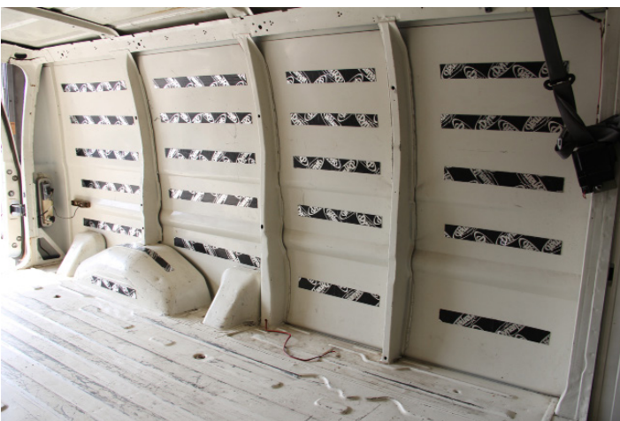
Typical Body Panel Sound Dampening and Barrier Insulation
