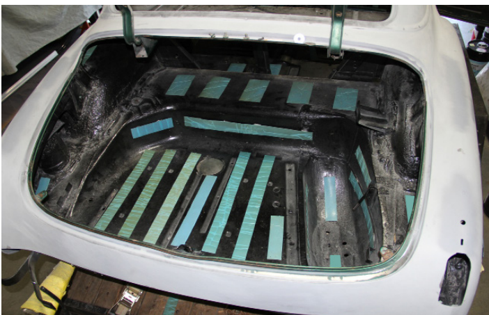
Typical Trunk Floor Sound Dampening and Barrier Insulation
