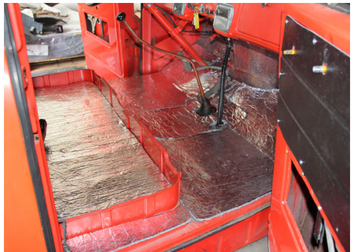
Typical Floor Panel Sound Dampening and Barrier Insulation
