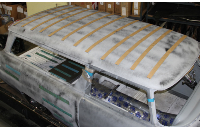
Typical Roof Panel Sound Dampening and Barrier Insulation
