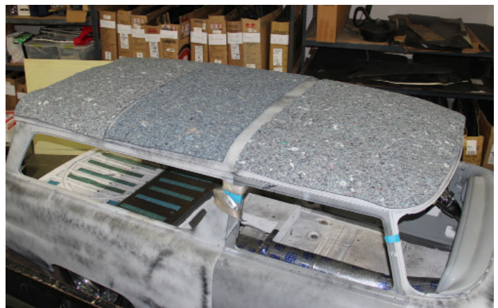
Typical Roof Panel Sound Dampening and Barrier Insulation
