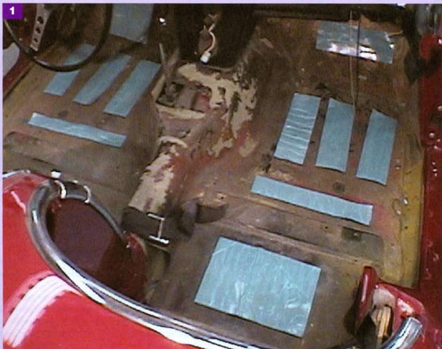
As seen in this photo, it is not necessary to completely cover the surface. Photos courtesy of Quiet Ride Solutions
