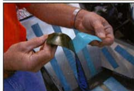
Dynamat is made of rubber and asphalt, which can reduce vibration by as much as 90 percent, according to Quiet Ride Solutions. This material has self-adhesive on one side, so you simply peel off the backing tape, and press into position with a roller.
