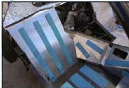
Start by loosely laying out the strips of Dynamat. You don't need to cover every square inch of the cockpit. It's sufficient to have spaces between the strips to break up the sound vibrations. The blue tape covers the self-adhesive side, so these strips will be turned over later on and pressed in place after determining their correct location, as indicated in the instruction sheet.
