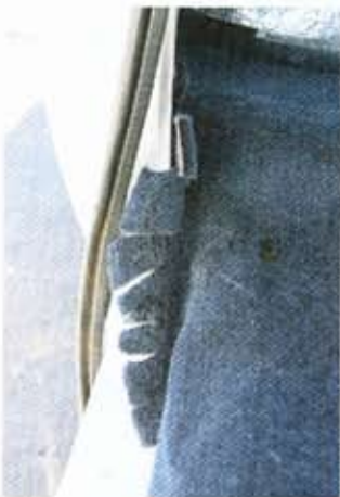
21 Notice how vertical slits were cut into the edges of the carpeting to make them pliable enough to tuck in. This step is critical to producing professional results.
