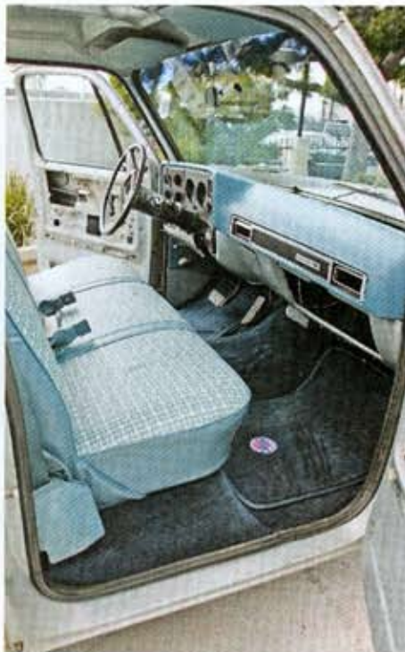
24 From start to finish it took Mario about two hours to install the TrimParts molded carpeting kit—double that time for a greenhorn.
