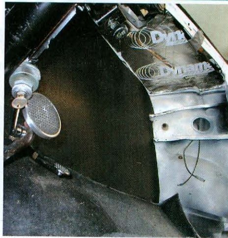
9) We installed the insulator using 1-inch-long tubular-threaded fasteners found at Home Depot. The ABS plastic upholstery-panel-based insulators are backed with AcoustiShield and embossed with exact factory-texture detail. It looks great as is, or it can be painted or covered with carpet.
