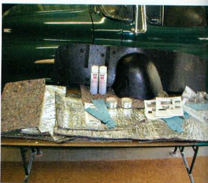
13) A typical AcoustiShield kit consists of pre-cut pieces of Heat Shield, strips of Dynamat, spray adhesive and foil tape. This one is for a '57 Chevy pickup and includes the optional fire-wall insulator. The step-by-step instructions show exactly where everything goes in your specific vehicle.
