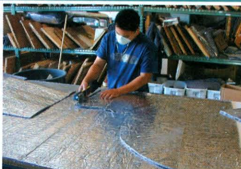
22) Here is where the patterns become kit pieces. Miles of insulation cross this table each week. A special cutter from Bosch makes cutting the tough material a snap.
