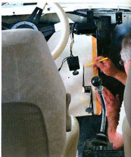
7) The best way to make just about any cutout is to first mark a pattern on cardboard, cut the hole, put it in place and trim to fit.
