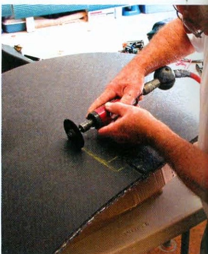
7) The best way to make just about any cutout is to first mark a pattern on cardboard, cut the hole, put it in place and trim to fit.
