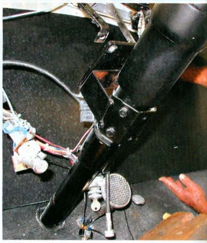
6) The insulator was a perfect fit. You can order it with or without factory holes. Ours is without holes. The only interference we ran into was the throttle pedal.
