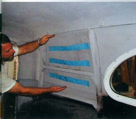
16) Before he started the top, Cox explained the Dynamat damping philosophy by taping three strips to the blank wall. A flat area of sheetmetal will "ring" or vibrate like a drum top, producing interior noise. Spreading equally spaced strips across the panel absorbs the vibration and cancels out the sound. Any seam or bodyline pressed into the panel, as well as curved sections, will have the same effect.
