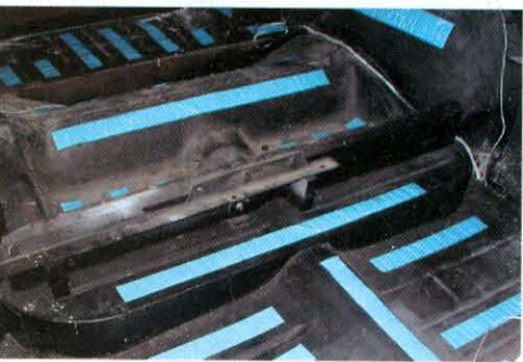
19) This is the rear-seat floor area, done the same way. People have been known to completely cover the inside of a car with Dynamat, usually in a quest for perfect audio acoustics. If they did, they spent way too much money and effort and added considerable weight to the car. The coverage you see here is all that's needed.
