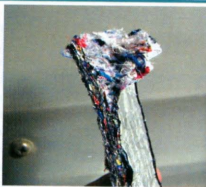
12) Here's a close-up look at the Quality Heat Shield insulation. What may look like ground-up rags and carpet is actually called "needle-punched synthetic fiber," a high-tech name for ground-up rags. It is very tightly bonded (we had to use pliers to pull this apart) to two layers of aluminum sandwiching and a fiberglass web for strength. This results in a thermal rating of R-18.3, the same as 6 inches of house insulation.
