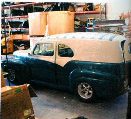
14) The first step in creating a kit for our "FANTM 47" coupe delivery was laying out the Dynamat strips needed to cancel the drum effects of that very large top. You can see them cut to length on the top.
