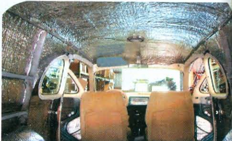
28) You've just gotta love a nice chrome interior! Especially when it is so effective in keeping your street rod as cool and quiet as a new Cadillac. We can't wait to get the interior built and the weatherstripping in so we can truly appreciate the new sensation.
