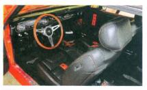
Brian added a few additional touches of his own during the interior upgrade, including fresh paint on the dash, a new Retrosound in-dash stereo with new Pioneer speakers and amplifier, and Lokar window cranks/door handles. A TMI one-piece headliner was installed as well and readers can look forward to a separate installation story on that in an upcoming issue.
