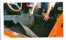
With the seats out of the way, Brian moves on to carpet removal. The carpet is retained by the rear quarter trim panels, door sill plates, and the kick panels. After removing these items, the carpet can be pulled up and removed.
