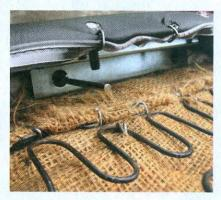
20 Install the new Sport XR foam and upholstery to the seatback following the same steps as previously outlined for the seat bottom. Use a long pick tool or scratch awl through the headrest bracket to locate the headrest guide locations and install the guides.
