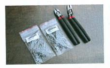
4 Upholstery work is all about getting the material in place and secured. It takes some arm and hand strength, a warm day (or careful use of a heat gun) to make the vinyl soft and pliable, and most importantly a pair of hog ring pliers and plenty of hog rings. These pliers and hog rings are from Eastwood. Expect to use 200-300 hog rings for a full interior set.
