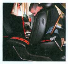
The final piece of the interior puzzle, the Sport XR front buckets, are set into place and secured with the original mounting hardware. TMI tells us that later this year you will be able to purchase completely assembled seats, saving the hassle of upholstery installation and dealing with old, cracked, broken, and rusty seat frames.
