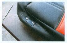
Use a pick tool or scratch awl to locate the seat back adjuster stop and reinstall it as shown. Use a razor blade to carefully cut the required holes for the two pivot pins as well.
