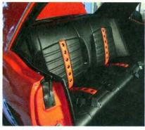
With the floor and trunk insulation complete, including a new insulated rear seat divider and insulation under the new vinyl wrapped TMI package tray, the freshly upholstered rear seat and vinyl wrapped quarter trim panels are reinstalled along with new premium cut pile carpet, also from TMI.
