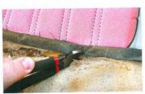
8 Remove the listing wires from the stock upholstery and slip them into the listing loops in the new TMI upholstery, then secure the new upholstery as shown. Pull the upholstery down over the seat bottom frame and adjust as necessary to ensure it is straight before securing with more hog rings.
