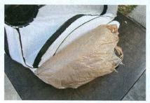
16 To work the upholstery over the larger Sport XR bolsters, a section of plastic (trash bags or grocery bags work perfect for this) is placed over each bolster, which allows the upholstery to easily slip over the foam instead of being grabbed by it.
