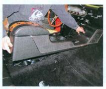
Once the front carpet is installed along with new speaker kick panels and the original door sills, the new TMI full length console is laid into place. The front of the console wedges nicely under the dash and at the rear we fastened a small bracket inside the console to secure it to the floor pan. The console features large cup holders, a front storage bin, and a rear storage cubby with armrest.
