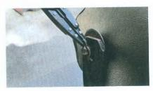
10 Remove the seat side shield/pivot trim on the bucket seat and disengage the pivot pins so the seatback and bottom assemblies can be separated. It is easier to separate them if you fold the seatback forward and use a large screwdriver or pry bar to separate the two halves.
