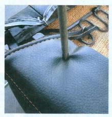
21 Locate the seatback cover retaining holes and use a large Phillips screwdriver in a twisting motion to cut the upholstery away. Transfer your old retaining clips to the new TMI covers and snap them into place.
