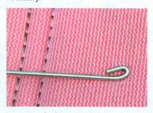
The new TMI Sport XR upholstery uses listing wires to secure the upholstery (just like the original seats), but the lengths are different. You'll be better off making new listing wires from wire rod (uncoated wire coat hangers work great), just make sure to put a small loop in the ends of the rods to prevent upholstery damage/poke through.
