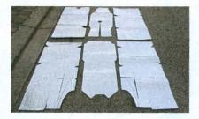
We also sourced QuietRide Solutions' AccoustiShield insulation kits for the floor, trunk, and body areas. Shown here is the floor kit. Each kit is incredibly complete with pre-cut insulation, sound dampening strips, spray adhesive, and foil sealing tape with fully illustrated instructions.
