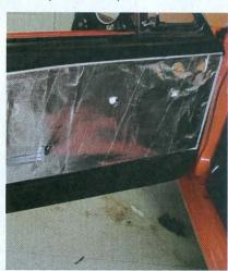
Before installing TMI's new full Sport X door panels, a QuietRide Solutions' WeatherShield kit was added. The WeatherShield kit includes sound dampener strips for the door skin and foil vapor/ moisture barriers for the door panel area.
