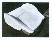
The new TMI Sport XR foam is cut to sit over the main seat frame hoop. There is no provision to hog ring the new foam to the seat frame, but it isn't really necessary.
