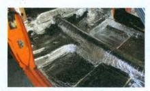
After the insulation sections have been glued into place, use the included foil tape to fully seal the edges of the insulation to the body and to cover all seams between the insulation sections.
