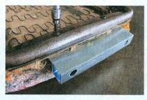
19 Moving on to the seatback, the upholstery and foam are completely stripped from the frame just as we did with the seat bottom. Adding TMI's optional headrest kit is a breeze at this point; simply cut away the burlap at the top of the seatback frame and bolt the headrest adapter into place as shown.
