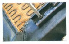
With the rear seatback and bottom completed, it is time to move on to the more complicated bucket seat upholstery work, which includes changing the foam. Begin your tear down by removing the seat tracks. Carefully remove the seat track return spring and then move the track slides as necessary to access the four retaining screws (per seat).
