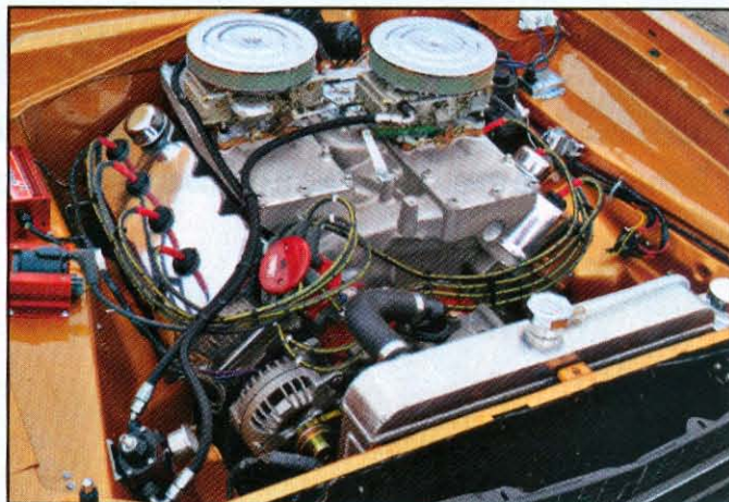
528-inch stroker Hemi pumped out a dyno'd 727 HP. Mill uses MP Megablock and Indy Legend Hemi heads. An all-aluminum street bullet is said to be in the works.
