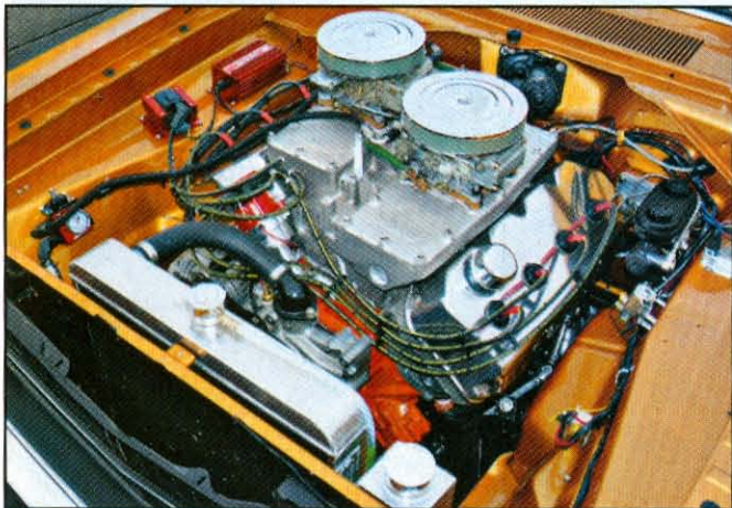
528-inch stroker Hemi pumped out a dyno'd 727 HP. Mill uses MP Megablock and Indy Legend Hemi heads. An all-aluminum street bullet is said to be in the works.
