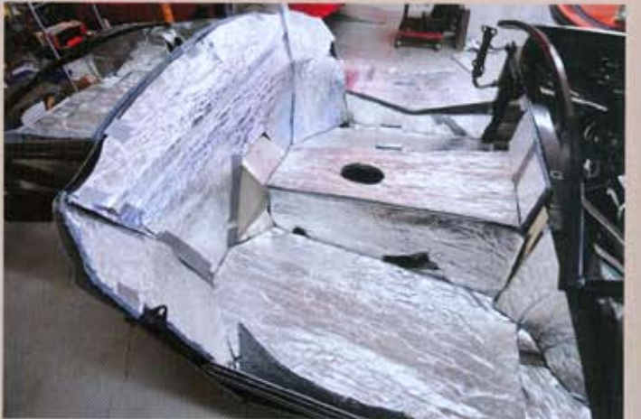
Be thorough, and cover as much of the interior area of the cockpit, firewall and trunk as possible.
