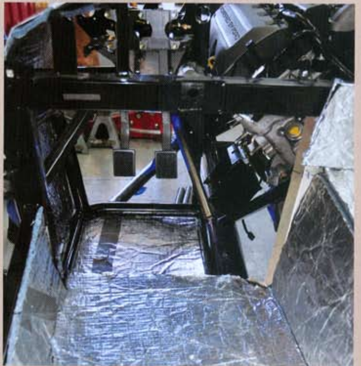
Note that sound can emanate from at least two different sources: via a solid material (the frame and body panels) and through the air (such as from the exhaust pipe, and somewhat surprisingly, the air intake as well). So we won't be stealing any thunder from the side pipes, just toning down the cockpit vibrations, such as in the footwells and under the seats.
