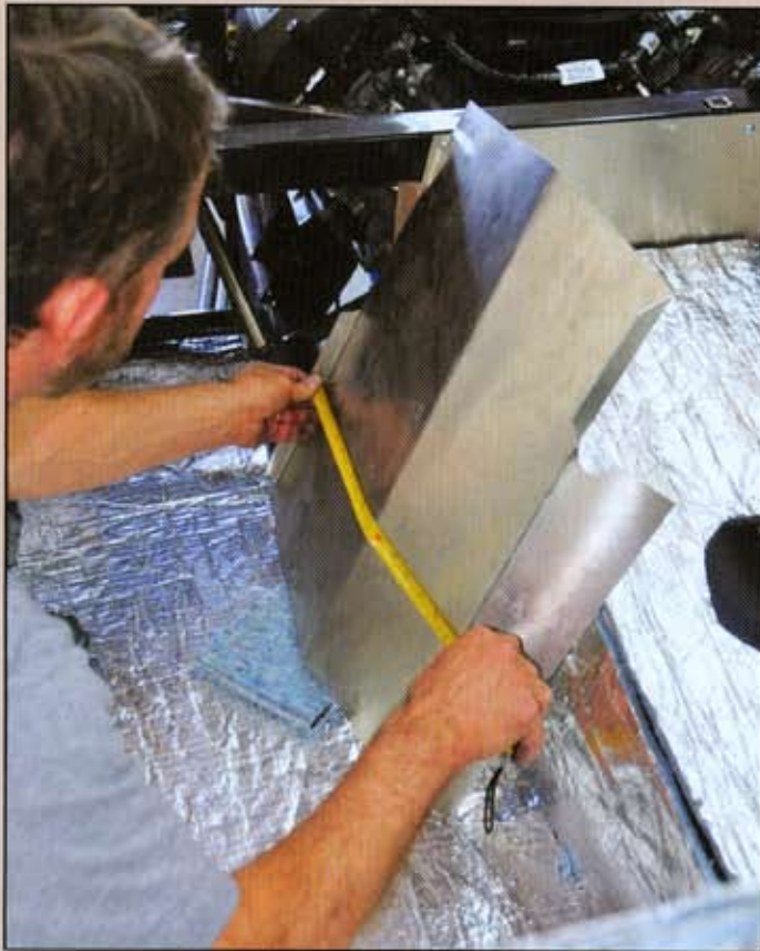
The FFR roadster kit includes a lot of separate aluminum inner panels, which can be measured or traced individually for the overall size of the pieces needed.
