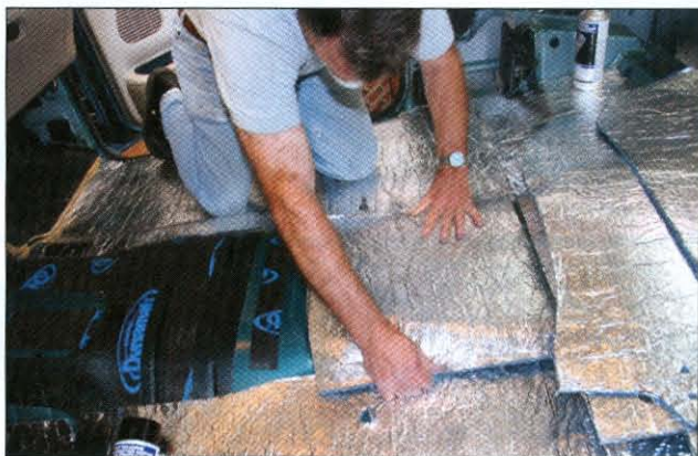
After adhesive is applied to both surfaces, put the Quality Heat shield on the Dynamat strips.
