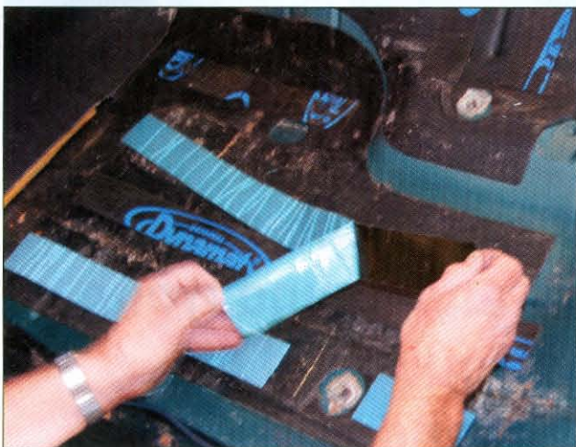
Then, simply press the Dynamat into position. Strips can work just as well as one solid sheet.
