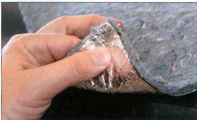
This close-up shows the top layer of reinforced aluminum foil and dense fabric padding.
