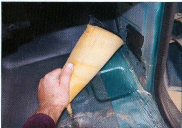
The factory insulation is pretty minimal, consisting of low-density foam in the foot wells and plastic bags filled with fiberglass wall insulation thrown into the rear quarters of the cabin.
