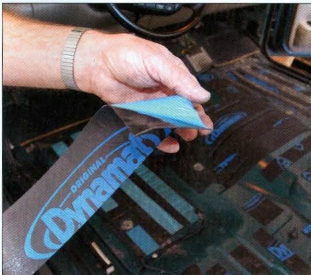
The blue backing tape peels off to expose the self-adhesive side of the Dynamat.
