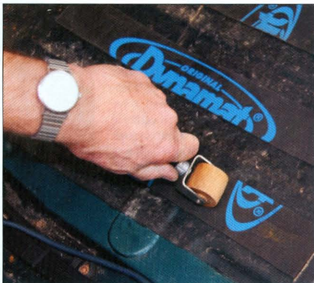
Use a roller to press the Dynamat strips in place so they bond tightly with the sheetmetal.
