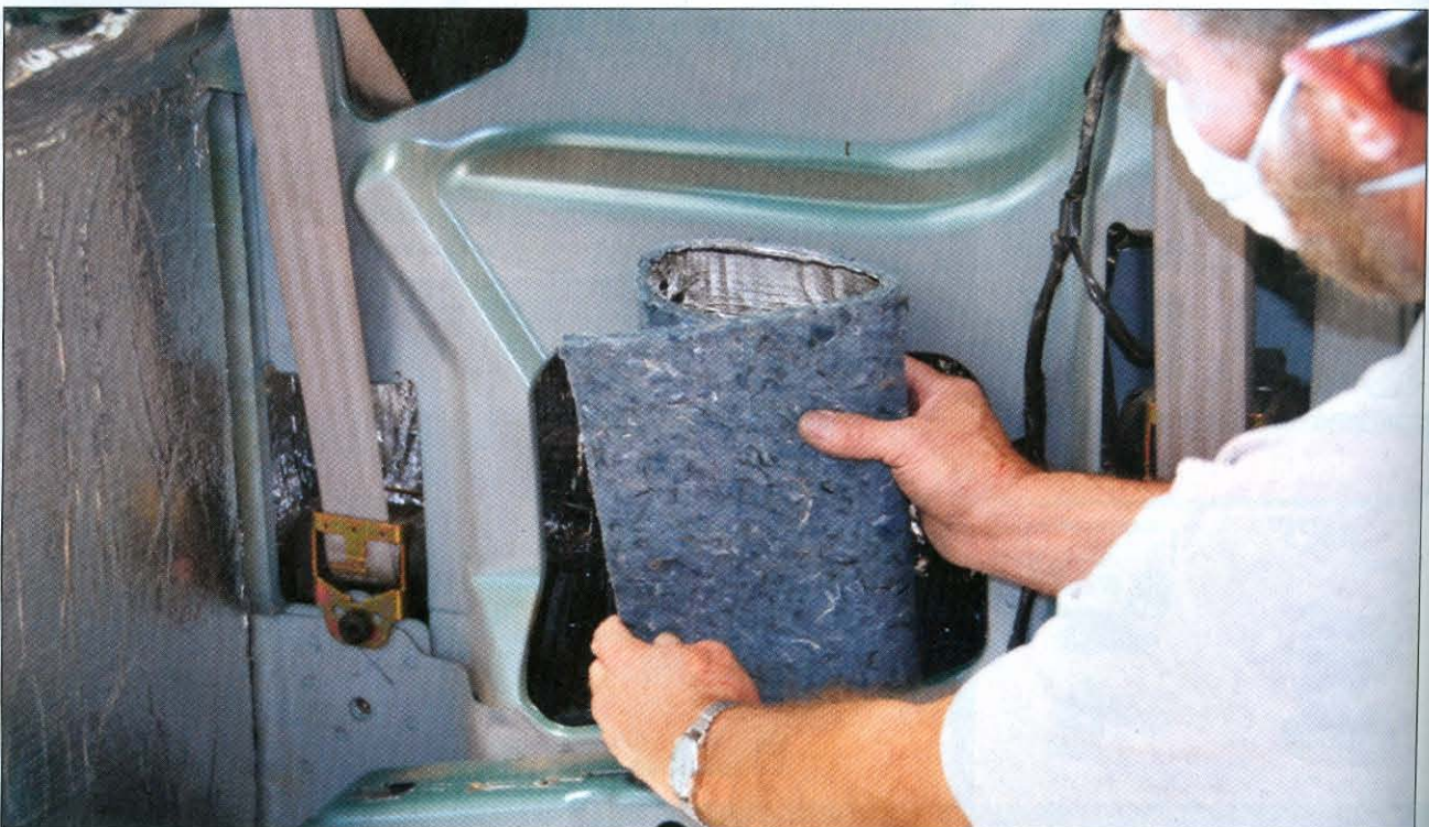
The insulation can be fitted into partially enclosed areas by folding it.
