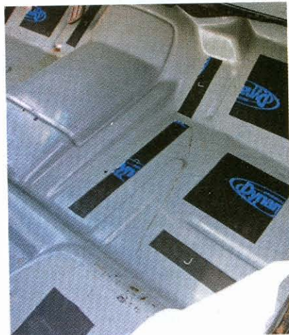
While installing the Quiet-Ride kit, we were amazed to discover the cab got quieter as the number of sound-canceling strips were applied.
