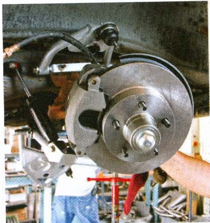
For front suspension, we used CPP tubular upper and lower control arms equipped with CPP F-44-type heavy-duty disc brakes. To upgrade standard C-10 disc brakes, this kit will bolt right on.
