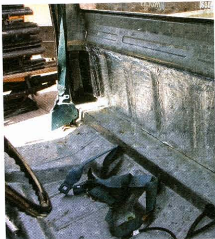
At a later date we will carpet the Big 10, but for Americruise, Quiet-Ride Solutions' foil-backed insulation held down the interior heat and noise quite well.
