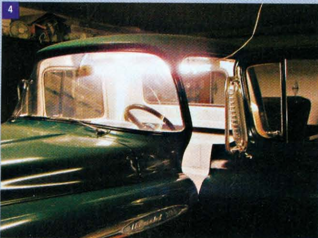
4 We hung a 4-foot two-bulb florescent light fixture from the headliner wiring, for a perfect light source that stayed out of the way.
